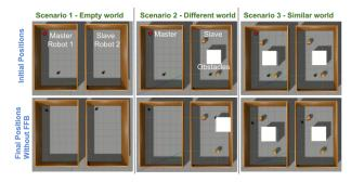
Fig. 2. Experiment setup of various scenarios simulated in ROS Gazebo. The red dot indicates the goal location set in the master side, which is running AMCL and *move\_base* planner. The Labor reacts to master's motion. The environment reaction Force Feedback (FFB) at Labor may be fed to the master.
